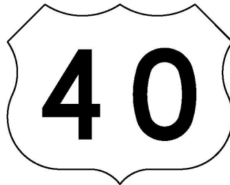
WHITE BACKGROUND WITH BLACK NUMERALS M1-4(G) (G) INDICATES SHIELD TO BE USED ON ALL GUIDE SIGNS AND DOES NOT REQUIRE BLACK BORDER
